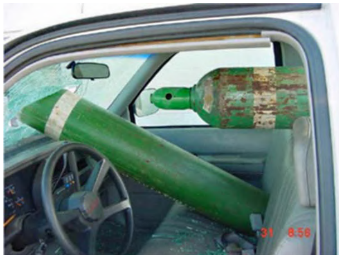
Damage from inappropriately stored and unrestrained cylinders in a vehicle, which stopped suddenly. Please note: Image is for illustrative purposes only. Cylinder colours do not comply with New Zealand Standards.
