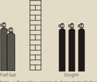
Note: wall must be a minimum of one metre higher than the tallest cylinder.
